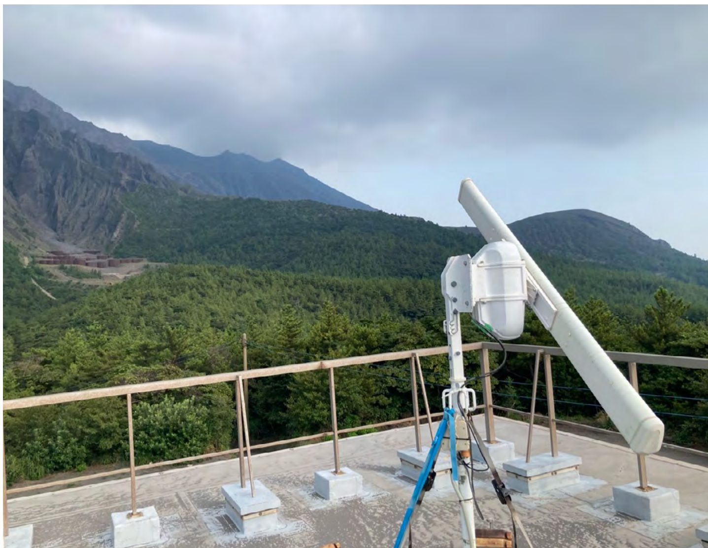
The shipboard radar installed at the Harutayama observation base ~3 km northwest of the Minamidake crater of Sakurajima. The radar was installed at close range to the crater so as to capture the detailed structure of the plume. The radar is set in 90° rotated position from the normal position in order to observe the detailed vertical structure inside the plume.
