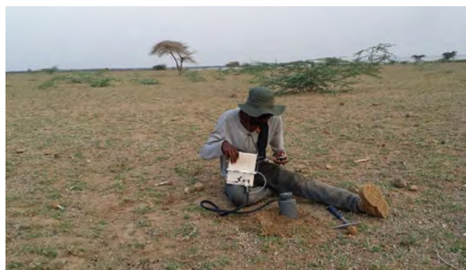
Amdemichael measuring soil CO 2 diffuse degassing around Fentale volcano in Ethiopia.
